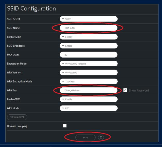
In both the 2.4Ghz and 5Ghz options, you will be able to change the WiFi name (SSID Name) and password (WPA Key). To prevent confusion, you will want to make sure the names and passwords are the same for both 2.4Ghz and 5Ghz. Press "Save" when finished.
