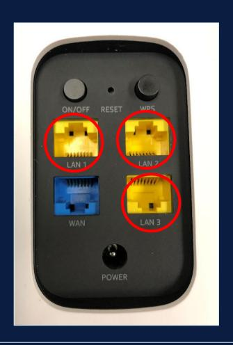
Connect a device to the router either wirelessly or through an Ethernet connection. If connecting through an Ethernet wire, make sure it is plugged into one of the LAN ports.
